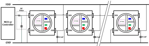
Note1: RC Filter must be added or reserved on the board for better waveform of signals in different applications. The value is subject to the practical system environment.
